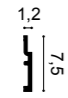
SX180 | SX180F HIGH LINE Duropolymer® 200 x 12 x 1,6 cm Designed by Pierre Daems
